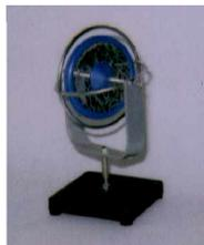
Stays stable in plane of rotation. No force off CG of wheel means no wheel plane displacement and very little precession except from frictional "cage" drag in bearings (possibly inertial drag from spatial arc travel of earth as to solar and galactic travel - causing extremely small wheel plane angular displacement.)
