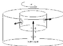
If water inflow in centrifugal water pump is created in axial direction and water outflow is made in radial directions the reaction force for this system is axial and unidirectional.
