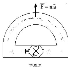
Some technical solutions were tested to prove efficiency of electrogravitation technology. One of them is so called T-shape capacitor. In classical plane capacitor the plates are in attraction but the forces are contradicted. In T-shape capacitor two electrodes are placed in the same flatness and both forces are co-directional forces.
